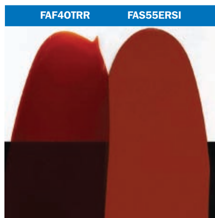
Figure 1: Drawdowns displaying the highly natural appearance of transparent iron oxide dispersions (left) versus a traditional colour dispersion (right).
